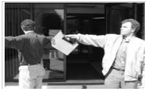
The Quantum Sniffer is a real-time, non-contact explosives trace detection device utilized to detect explosives vapors and particles from surfaces.
